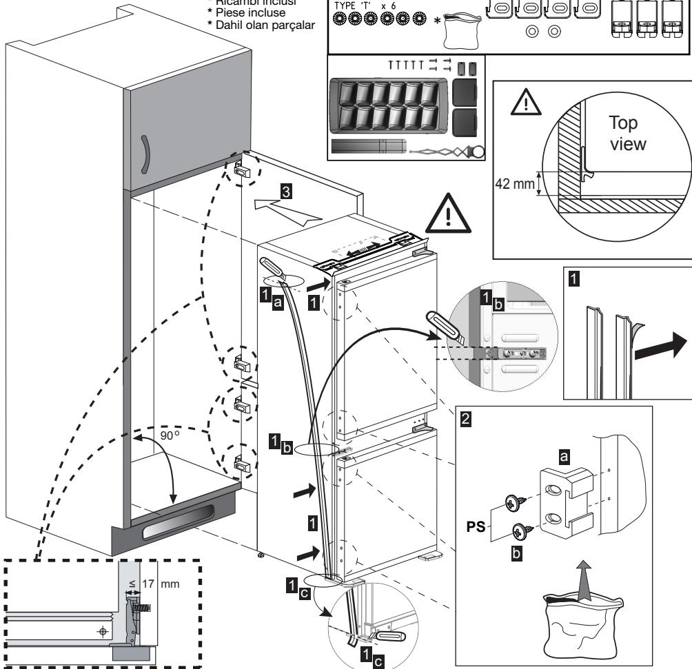
**Note:** Screws for connecting top plastic part should not be screwed very hard, because of moving the plastic part easily left or right side.
