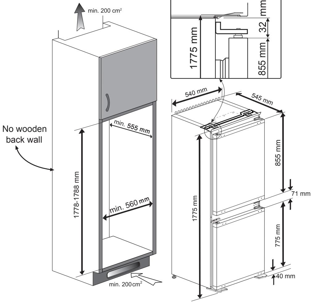
The back wall of the wooden cabinet must be left open completely to kitchen wall in order to allow sufficient air circulation to cool down the condenser unit for energy efficiency.
