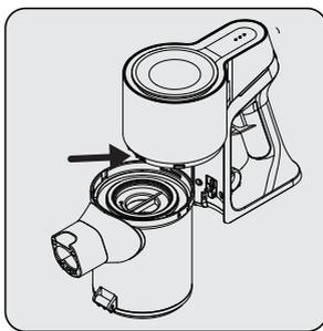
Fix the connector of dustbin to the holes on the body, then fix the dustbin until you hear the click sound.
