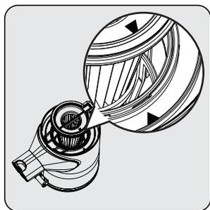
While placing the pre-filter, make sure that arrows on the pre-filter and the body are aligned.
