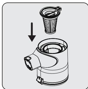
Attach pre-filter to the plastic filter back.
