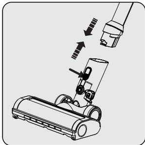
Press the electric turbo brush release button on the electric turbo brush and push it in the direction of arrow towards the tube.
