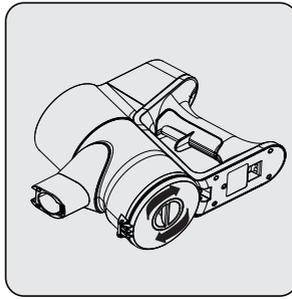
In order to operate the product at high performance for a long time, it may be necessary to clean the filter by rotating the mechanism under the dust container. It will help to clean the filter easily.
