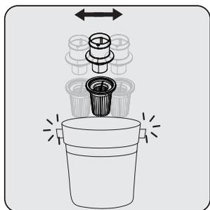
Remove the dust on the pre-filter and the plastic filter by tapping it on a hard surface such as a waste bin or by using a brush.
