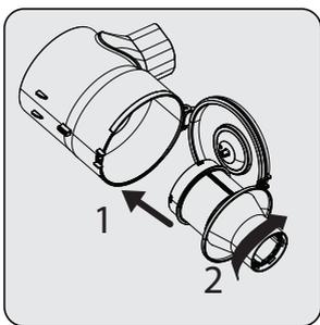
To insert the plastic filter, firstly place the plastic filter (1), then rotate it clockwise to lock it (2).
