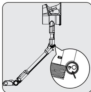
You can fold the tube for easy access to areas such as armchairs and under tables. You can fold the tube by pressing the round button mechanism on the left side that allows the tube to be folded.
