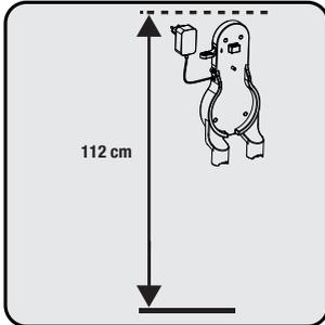
Position the charging dock at a height of minimum 112 cm from the ground.
