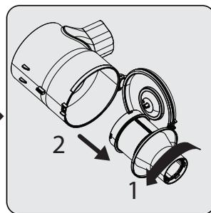
To take out the plastic filter, first rotate the plastic filter counter clockwise (1), then pull out the filter (2).
