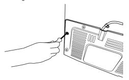
Attach 2 plastic wedges on the ventilation cover as shown in the figure.
