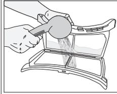
A layer can build up on the filter pores that can cause clogging of the filter after using the dryer for a while. Wash the lint filter with warm water to remove the layer that builds up on the lint filter surface. Dry the lint filter completely before reinstalling it.
