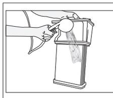
Clean the condenser by applying pressurized water with a shower armature and wait until the water drains.
