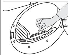
There are dampness sensors in the dryer that detect whether the laundry is dry or not.
