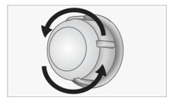
c. If your oven lamp is type (A) shown in the figure below, rotate the oven lamp as shown in the figure and replace it with a new one. If it is type (B) model, pull it out as shown in the figure and replace it with a new one.
