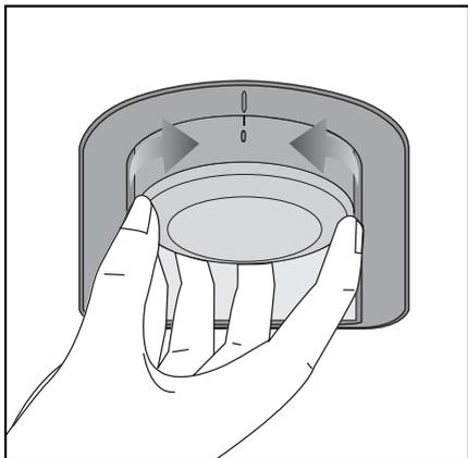
Operating temperatures are controlled by the thermostat knob (see diagram) located on the ceiling of fridge compartment. Settings may be made from 1 to 5, 5 being the coldest position.
