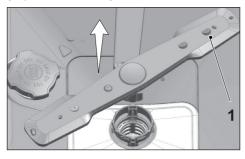
Check if the holes on the lower impeller assembly are clogged. If they are clogged, remove and clean the impeller assembly. (depends on model)
