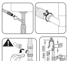
Drain pipe must be connected to the sewage system and it should not be connected to any surface water.
