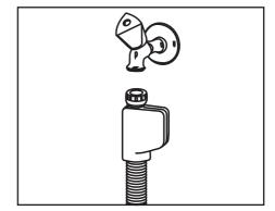
As the hose set contains electrical connections and assemblies, never shorten or lengthen the hose with extension hoses.
