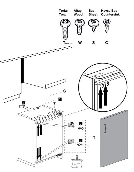
**Note:** For installation Step 1, the screws for the top plastic part should not be tightened fully to allow side to side adjustment.
