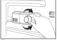
The operating temperature is regulated by the temperature control.
