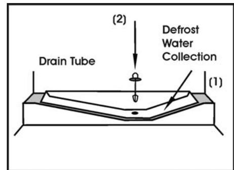
If, at any time, the defrost water does not drain from the collection channel, check that no food particles have blocked the drain tube. The drain tube can be cleared with a pipe-cleaner or Pushing the special plastic plunger provided down the drain tube (2).
