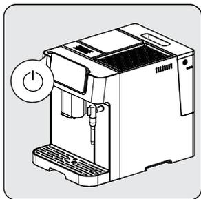
Switch on the appliance by pressing the power on/off button. The appliance turns on, starts pre-heating and auto-cleaning. It is ready for use in idle mode in which all icons are lit.
