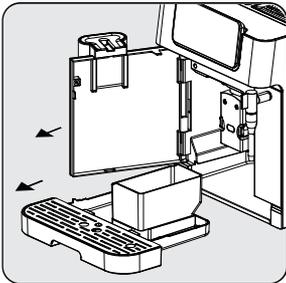
Open the front cover. Remove the drip tray and the coffee residual container.
