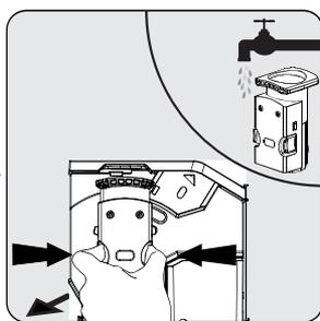
Remove the brewing unit. Wash with water and dry afterwards.
