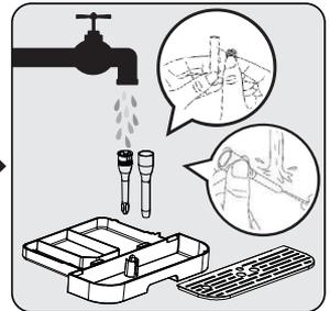
Empty the coffee residual container and the drip tray. Wash the metal tube with warm running water and use the needle or the bristles of the brush to clean the hole. Wash the nozzle cover with warm running water and use the needle or the bristles of the brush to clean the hole. Dry them afterwards.
