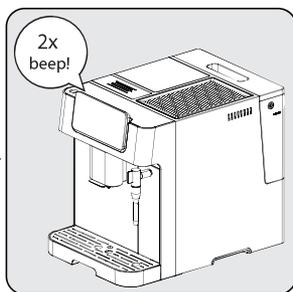
When the volume of coffee meets your desired volume, release the button. If you hear two beeps, that indicates the machine has saved this volume of coffee.
