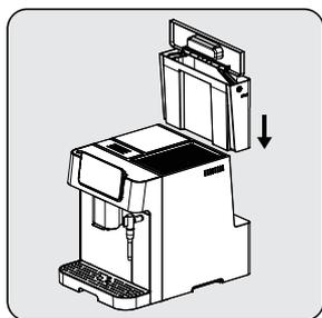
Place the water tank back in by using the lid as the handle.
