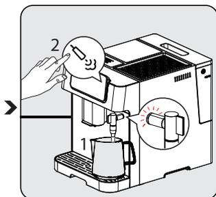
When the indicator lights are still, steam nozzle is ready for use. Place a milk filled cup or pitcher under the steam nozzle. Press the steam nozzle button again for starting the milk frothing, and stop by pressing again.
