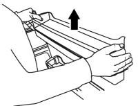
2. Hold both sides of the water tank and remove at 45° angle.
