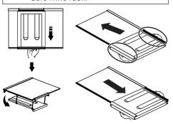
To group the wine rack, first remove the glass shelf from the refrigerator. Place it on the glass shelf by pushing the plastic part through the front and back grooves as shown in the picture. The product will be ready to use with the foldable wine rack. To remove the foldable wine rack, first remove the glass shelf from the refrigerator. Then grab the plastic part and pull it in any direction. You can now use the product without a foldable wine rack when needed.
