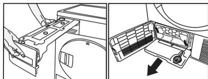
2. Drain the water in the tank.
