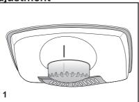
Operating temperatures are controlled by the thermostat knob (see diagram) located on the ceiling of fridge compartment. Settings may be made from 1 to 5, 5 being the coldest position.
