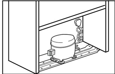
**IMPORTANT:** Care must be taken” while cleaning / carrying the appliance to avoid touching the bottom of the condenser metal wires at the back of the appliance as you might injure your fingers and hands
