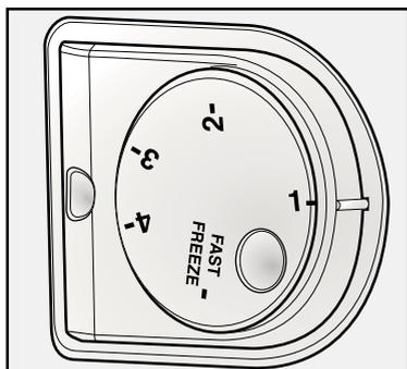
Operating temperatures are controlled by the thermostat (see diagram) located on the inner side wall of the freezer compartment. Settings may be made from 1, 2 ... fast freeze, fast freeze being the coldest position.
