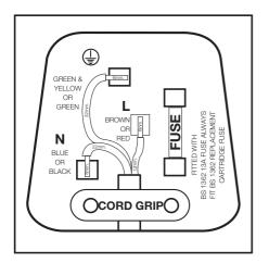
an ASTABEAB approved BS 1362 fuse of the same rating must be used. Do not forget to refit the fuse cover. In the event of losing the fuse cover the plug must not be used until a replacement fuse cover has been fitted. Colour of the replacement fuse cover must be the same colour as that visible on the pin face of the plug. Fuse covers are available from any good electrical store.
