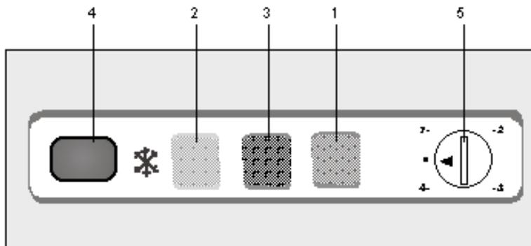
Temperature is controlled by the thermostat which is located on the rear wall of the cabinet (see the diagram on page 5). Thermostat knob is located on the indicator light set. “Number 4” is the coldest setting (see the diagram on page 8).
