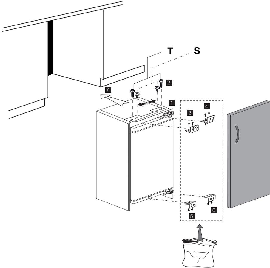
**Note:** Installation step for 2, screws for connecting top plastic rpart should not be screwed very hard, because of moving the plastic part easily left or right side.
