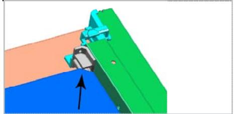
When installing the innermost glass panel (1), make sure that the printed side of the panel faces towards the inner glass panel. It is important that the lower corners of the innermost glass panel are seated into the plastic slots.
