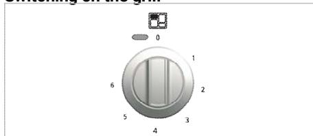
Turning the Grill control knob clockwise provides various levels of grilling.
