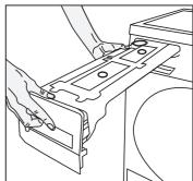
Drain the water in the tank.
