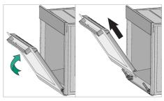
Pull the removed door upwards to release it from the right and left hinges and remove it.
