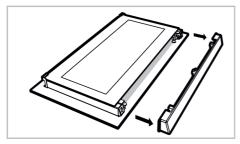
As shown in the figure, gently lift the innermost glass (1) towards "A" and then, remove it by pulling towards "B".
