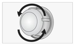
3. If your oven lamp is type (A) shown in the figure below, rotate the oven lamp as shown in the figure and replace it with a new one. If it is type (B) model, pull it out as shown in the figure and replace it with a new one.
