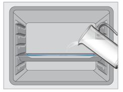
Set the oven to the easy steam cleaning operating mode and operate it at 100°C for 15 minutes.
