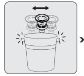
Remove the dust on the plastic filter by tapping it on a hard surface such as a waste bin or by using a brush.
