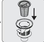
Attach EPA E10 filter to the plastic filter back.
