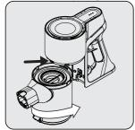
Fix the connector of dustbin to the holes on the body, then fix the dustbin by turning counterclockwise until you hear the click sound.
