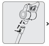
Push the tube (10) in the direction of arrow towards the body by pushing on the tube release button (6).
