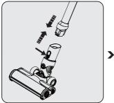
Press the electric turbo brush release button (11) on the electric turbo brush (12) and push it in the direction of arrow towards the tube.
