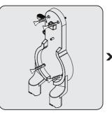
1- Fix four dowels (18) on the wall 2- Place four screws (17) into their locations on the charging dock (8) and mount on the dowels on the wall.
