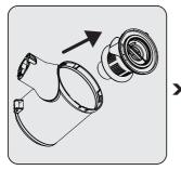
Pull EPA E10 and plastic filter holding from the EPA E10 handle.
