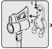
1- Push the appliance release button (7) on the charging dock (8) downward and pull the appliance towards yourself at the same time. 2- Remove the appliance from the charging dock (8).
