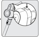
To switch to the maximum power when operating in the minimum power, push the power adjustment button (2). To switch to the minimum power when operating in the maximum power, push the power adjustment button (2) again.
