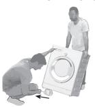
Tilt the machine backwards to remove the packaging reinforcement. Remove the packaging reinforcement by pulling the ribbon. Do not make this operation alone by yourself.
