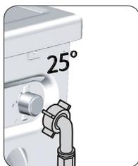
Tighten all hose nuts by hand. Never use a tool when tightening the nuts.
