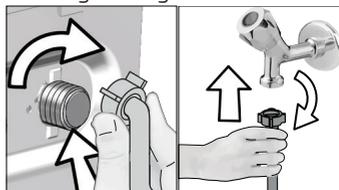
Open the taps completely after making the hose connection to check for water leaks at the connection points. If any leaks occur, turn off the tap and remove the nut. Retighten the nut carefully after checking the seal. To prevent water leakages and damages caused by them, keep the taps closed when the machine is not in use.
