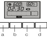
Some functions cannot be selected together. If a second auxiliary function conflicting with the first one is selected before starting the machine, the function selected first will be canceled and the second auxiliary function selection will remain active. For example, if you want to select Quick Wash after you have selected the Prewash, Prewash will be canceled and Quick Wash will remain active.
