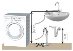
• Connect the drain hose to a minimum height of 40 cm and a maximum height of 100 cm.
