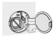
Open the pump filter cap.
