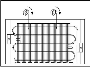
**3.** Fit the two plastic wall spacers supplied with the appliance on to the condenser at the back of the refrigerator by rotating 1/4 turn (see diagram).
