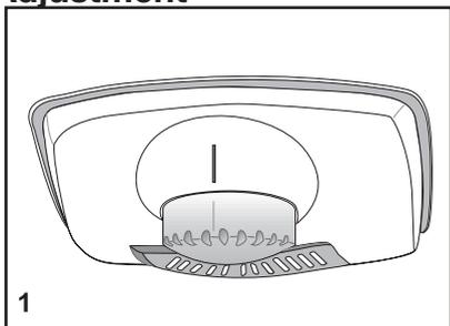
Operating temperatures are controlled by the thermostat (see diagram) located on the ceiling of fridge compartment. Settings may be made from min to max, max being the coldest position.
